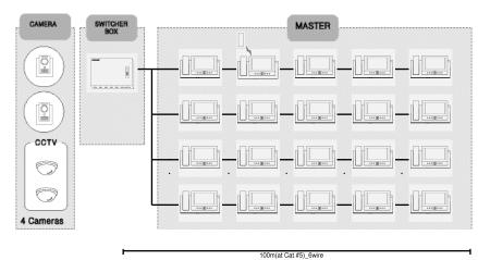
Maximum connect with up-to 4<sup>th</sup> cameras \*Available to connect with CCTV camera Maximum connect with up-to 20<sup>th</sup> monitors
